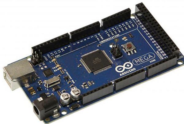
Figura 2. Arduino MEGA.
