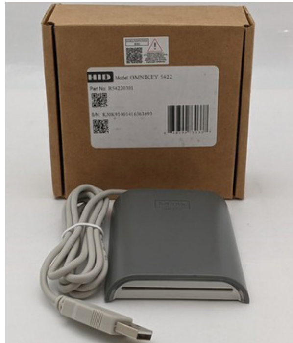
Figura 4. Lector HID OMNIKEY 5422 Dual Interface.
