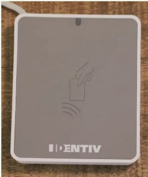
Figura 3. Lector Identiv uTrust 3700 F Contactless.
